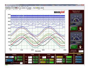
**Typical Screen:** Above is a typical screen with 10 channels of analog data and 8 bits of digital data being plotted along with two meters that can display any of the analog or digital data.
