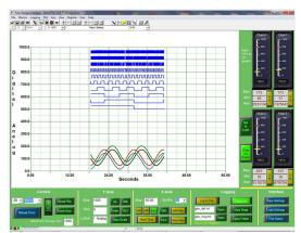
**MakerPlot** is Windows® software for plotting analog and digital data generated by your microcontroller.
